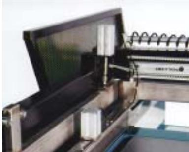
An accurate adjustable lift-off system is very important for printing large sizes. The lift-off system of the Vipro Horizon Mk-II is driven by a separate pneumatic circuit so it can lift accurate and steady, free from the movement of the squeegee carriage. The screenholders can be adjusted independently up to the maximum screensize; standard they have a quick locking system. As an option pneumatic locking of the screens is possible.
